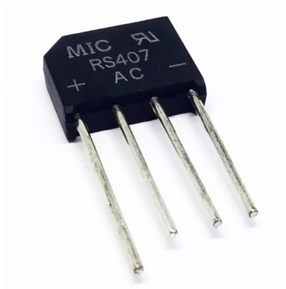
Figure 07.10: rectifier bridge – here we have an IC.
