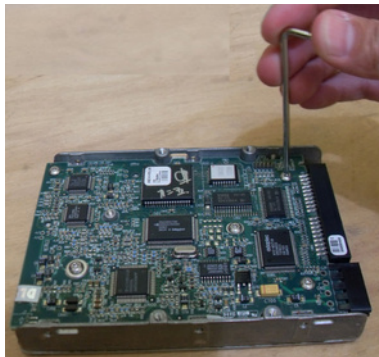
Figure 04.13: removing a screw from a HD with a torx key.
