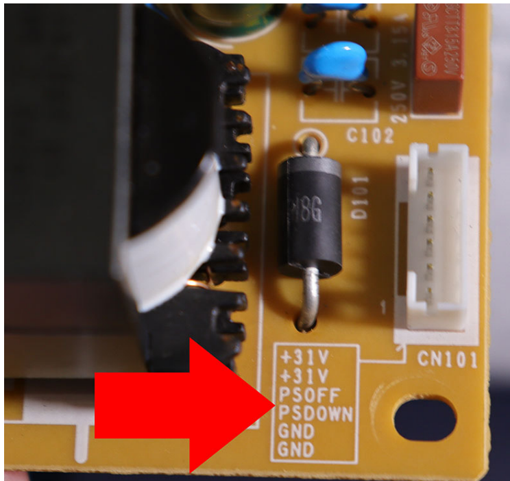
Figure 06.9: table with voltages of each pin from the logic board power connector.
