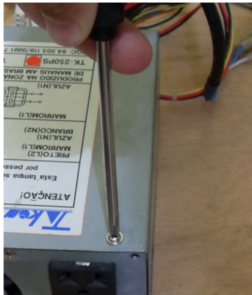
Figure 04.10: removing the screw from a source with a Phillips screwdriver.
