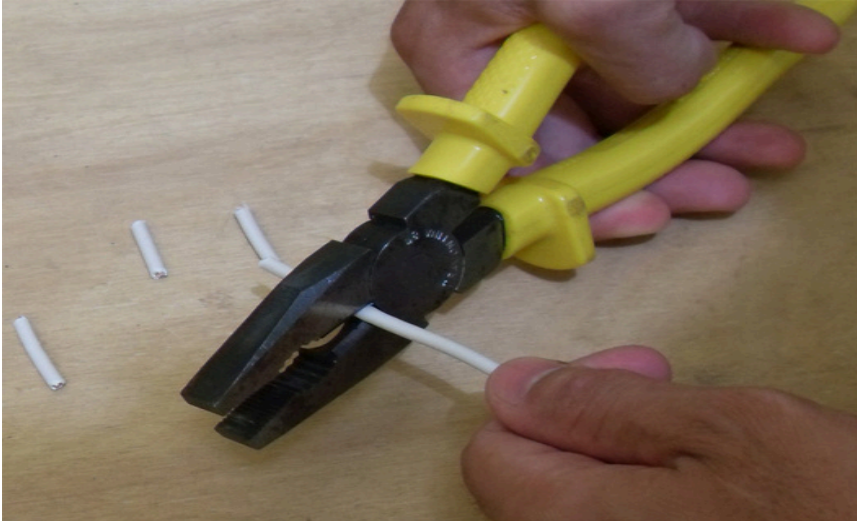
Figure 04.2: when using pliers, the force applied to the handle is transferred to the head
