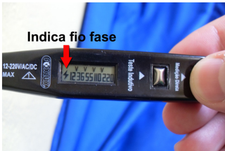
Figure 04.24: phase wire located
