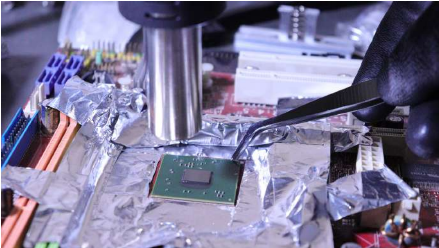
Figure 04.12: checking if the chip is loose. Give it a little push to the side.
