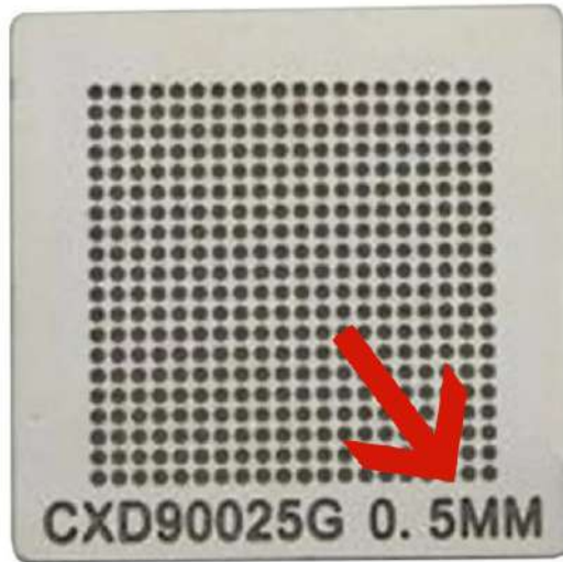
Figure 04.28: diameter of the sphere. In this example is 0.50mm.
